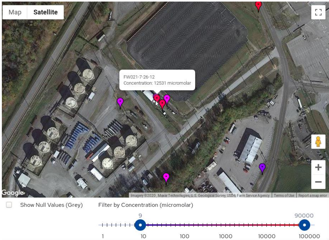
Figure S-4D: An example of the map resulting from Figure S-4C, in which the concentration of nitrate from several samples is plotted on a map, according to the sampling location.
